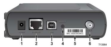
1 POWER – Connects the cable modem to the 12 VDC output of the AC power adapter that is provided with your cable modem
